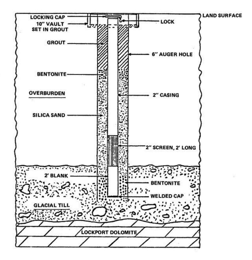
Figure 15. Completed Shallow (Overburden) Well.
