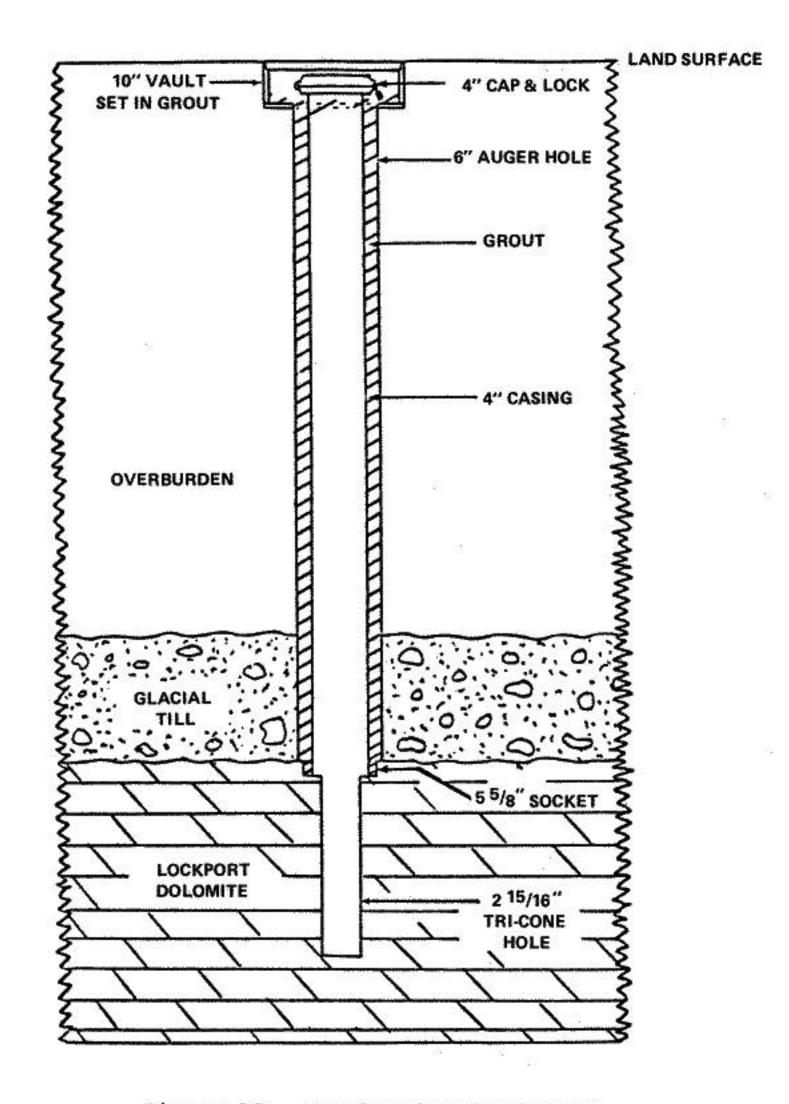
Figure 16. Completed Bedrock Well.
